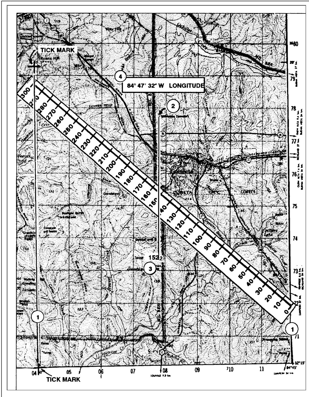
Figure 4-5. Determining longitude.
