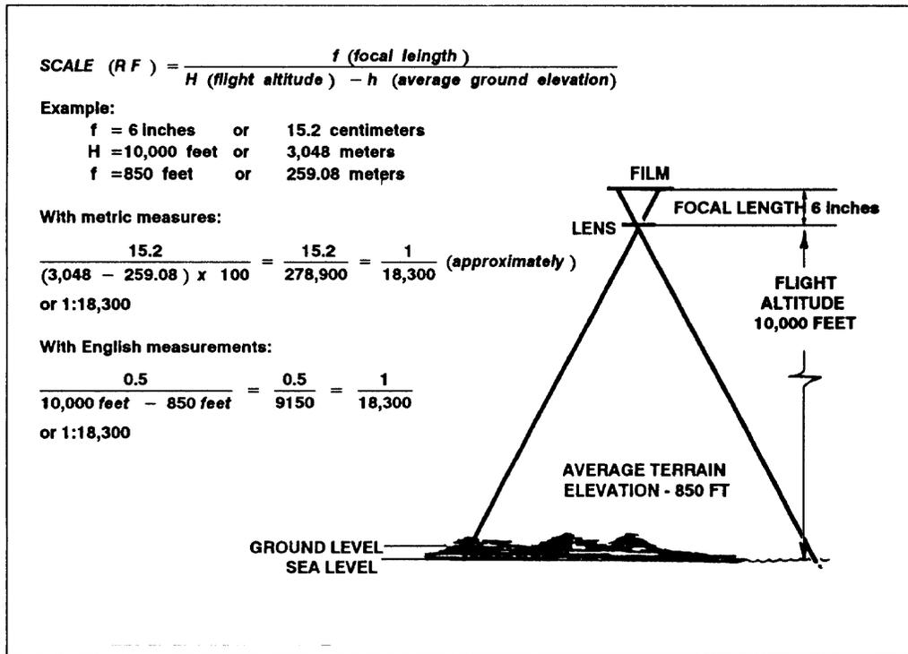
Figure 8-9. Computation of scale from terrain level.
