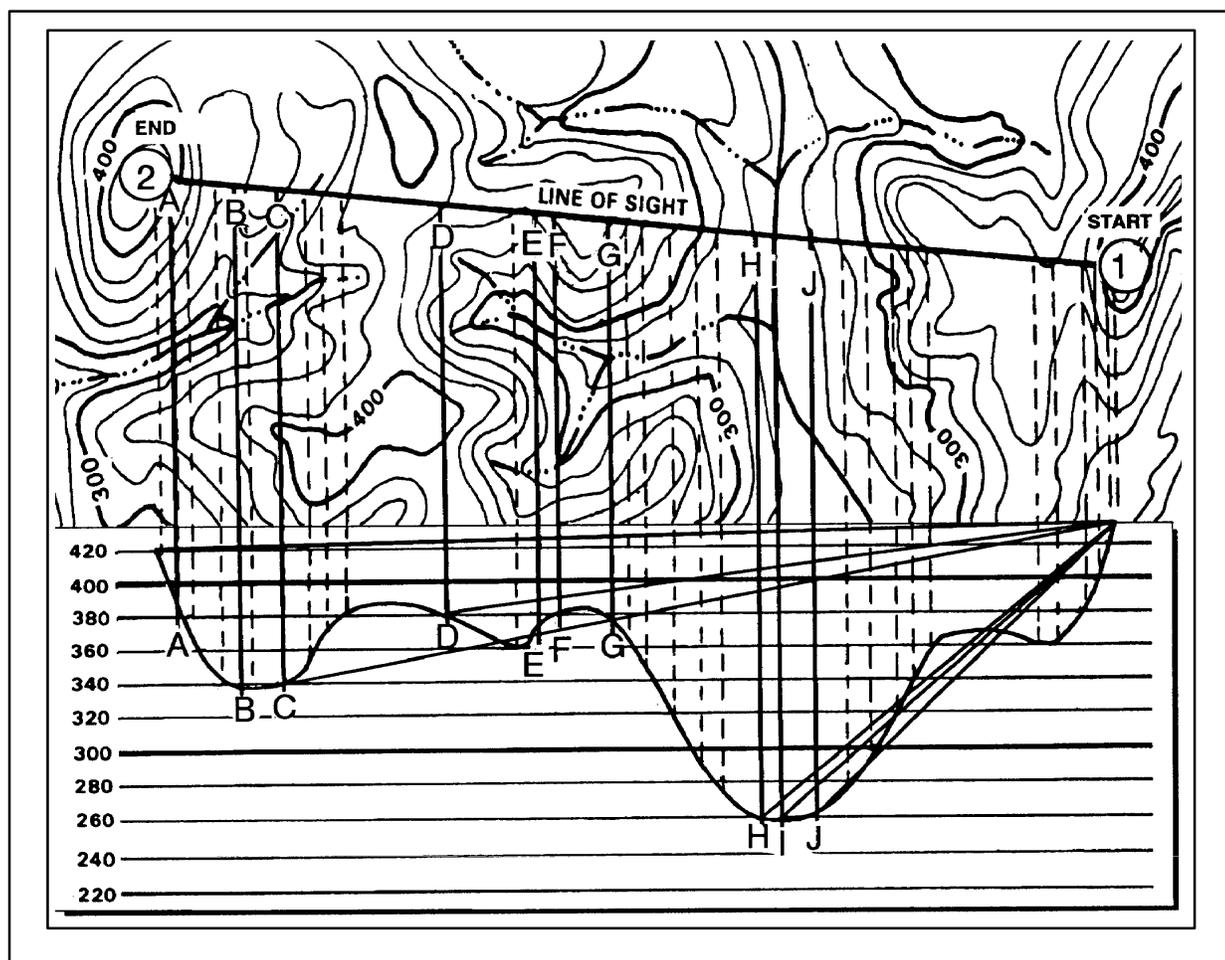
Figure 10-30. Drawing lines to additional points.
