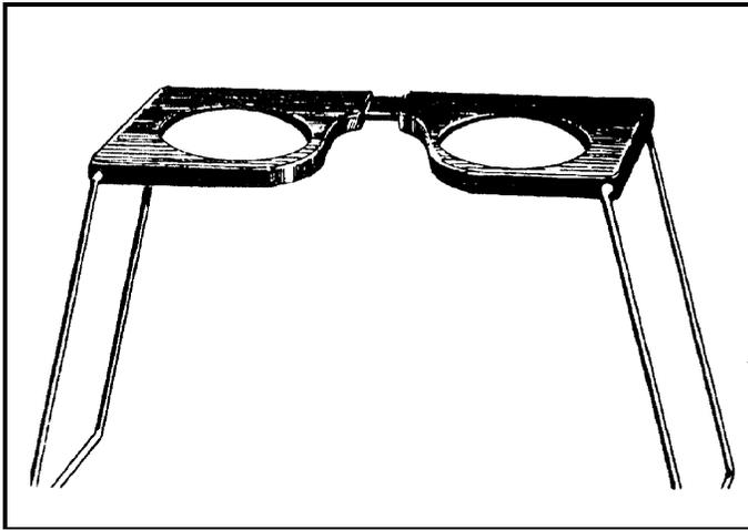
Figure 8-22. Pocket stereoscope.
