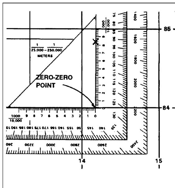
Figure 4-16. Placing a coordinate scale on a grid.
