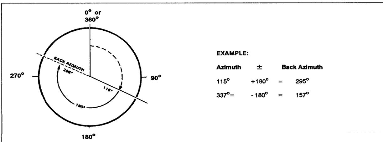
Figure 6-3. Back azimuth.
