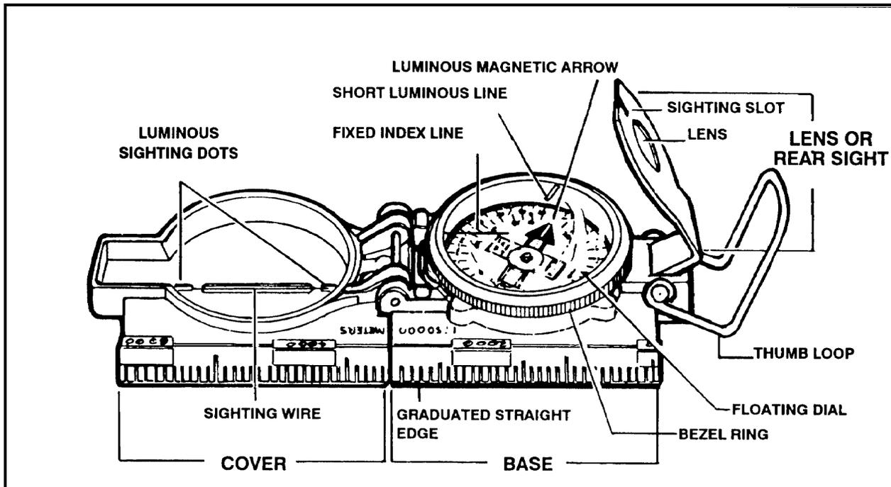
Figure 9-1. Lensatic compass.
