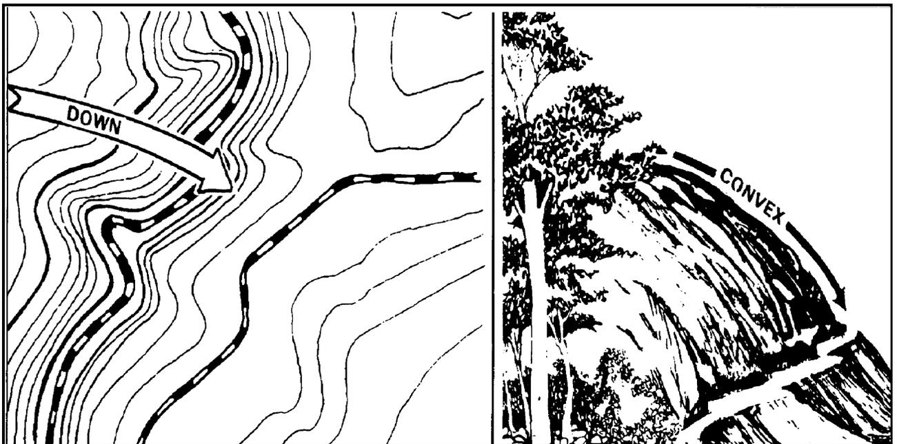
Figure 10-9. Convex slope.
