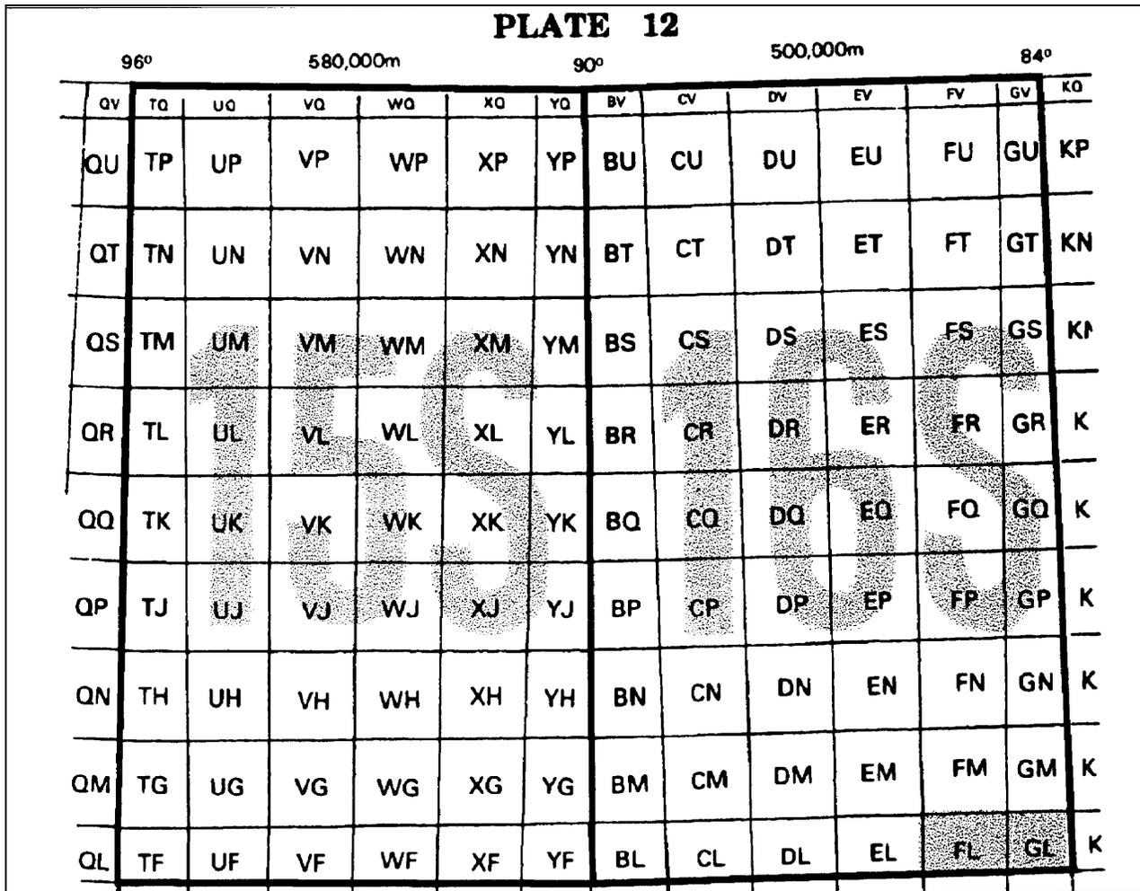
**Figure 4-11. Grid zone designation and 100,000-meter square identification.**
