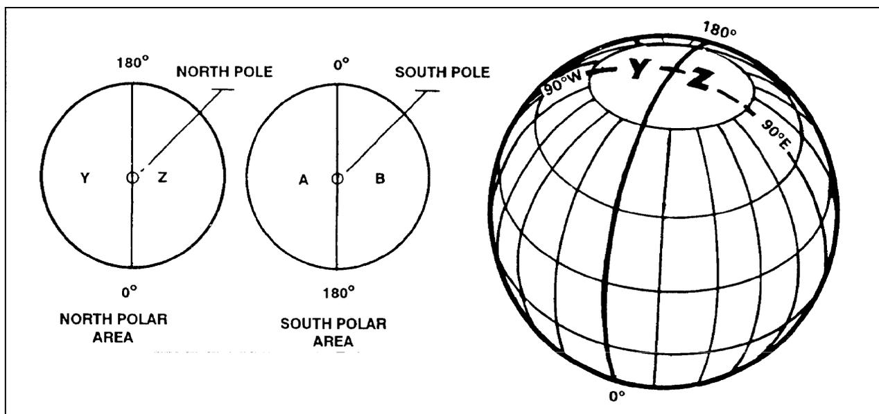
Figure 4-10. Grid zone designation for UPS grid.
