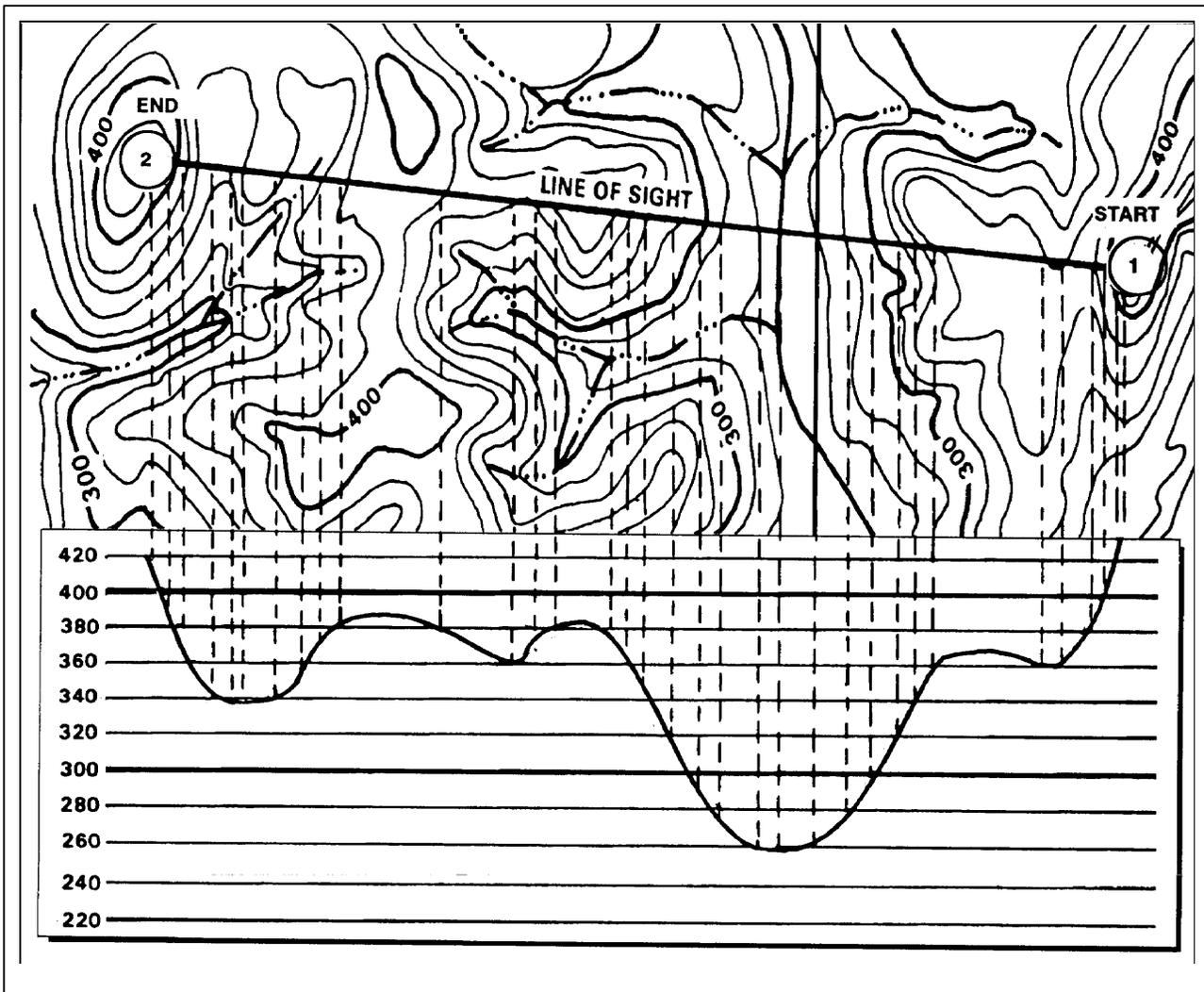
Figure 10-29. Dropping perpendiculars.
