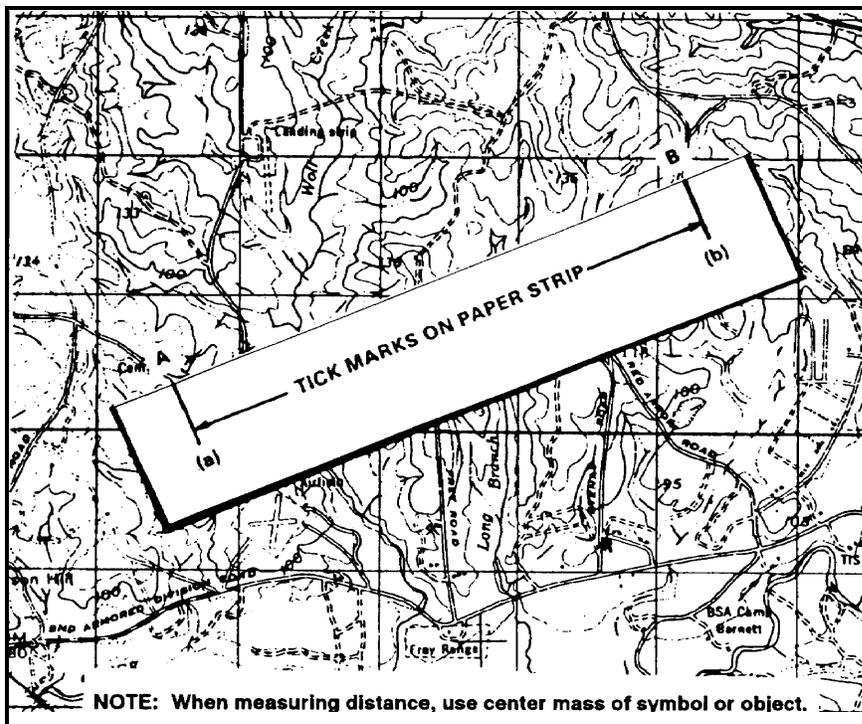
Figure 5-3. Transferring map distance to paper strip.
