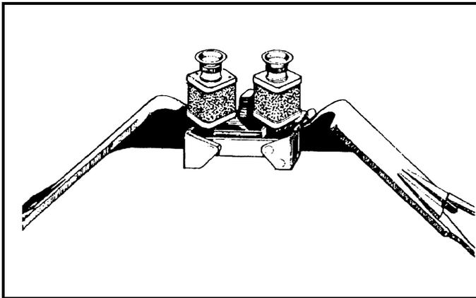
Figure 8-23. Mirror stereoscope.
