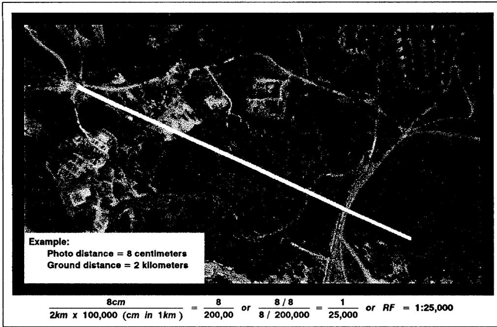
Figure 8-8. Selection of points for scale determination.
