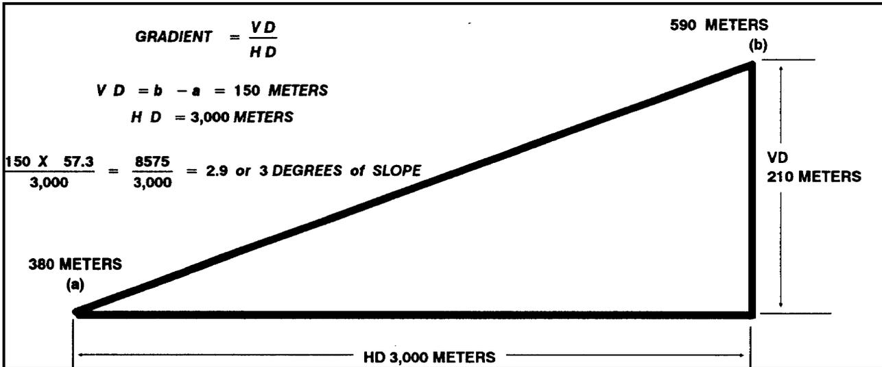
Figure 10-14. Degree of slope.
