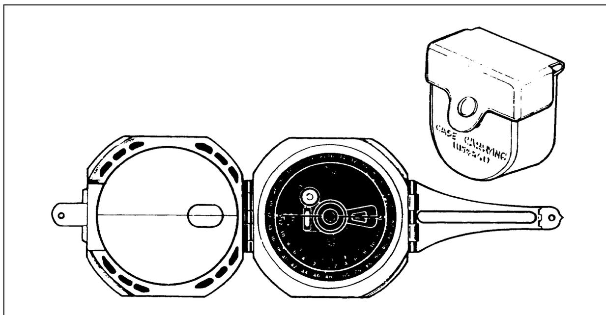
a. **Reading the Azimuth Scale.** Azimuths are read from the azimuth scale from the black end of the compass needle.
