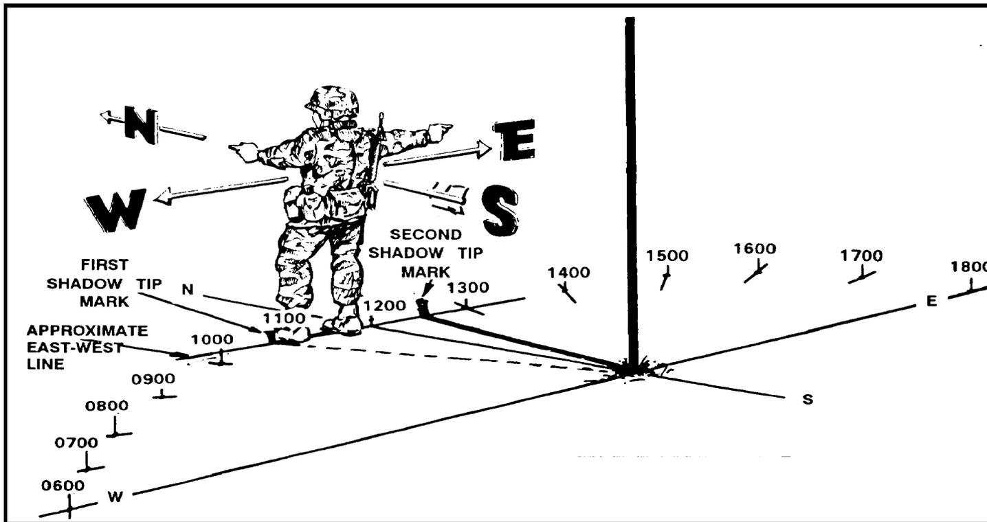
**Figure 9-7. Determining directions and time by shadow.**
